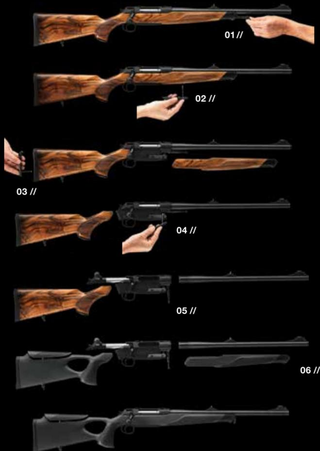
Backpack-sized in a trice: Whether you need to reach the hunting area on foot or come down the mountain with a chamois in your rucksack, it only takes a few seconds to remove the buttstock with the SUS and reduce the size of the S404 with 51 cm (20 in) barrel to an impressively packable 69 cm (27 in) overall. The S404 can traverse the most rugged trail yet can go from portable to shootable in moments.
