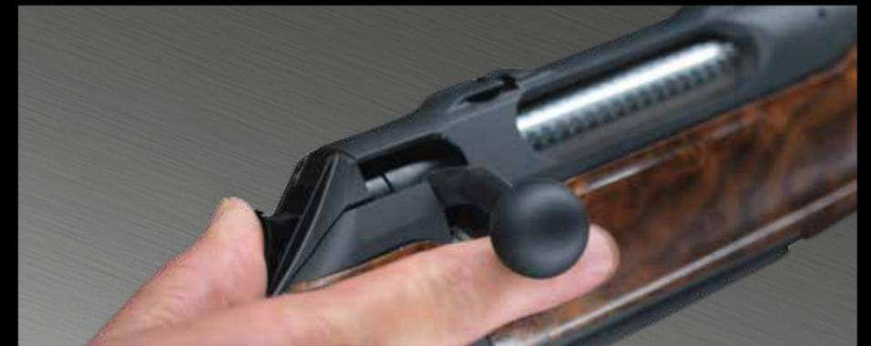
Good enough isn't enough: In addition to the manual cocking feature, an automatic firing pin safety works inside the S404 to prevent it from firing when the bolt is not fully closed. In order to open the bolt with the gun on safe – e.g. to load and unload – it is only necessary to push the cocking slide forward two millimeters while at the same time lifting the bolt handle. This way, safe handling becomes instinct aided by intelligent technology.
